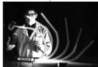
A researcher demonstrates the flexibility of a bendable heat pipe.
