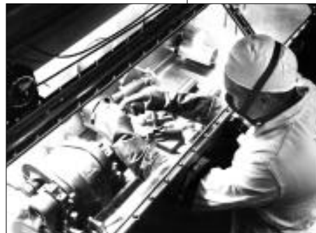
A worker handles special nuclear materials in a glove box at the Laboratory's plutonium processing facility.
