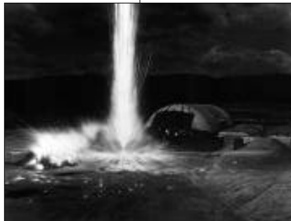
A dynamic test at the PHERMEX facility of a weapon design using conventional explosives but mockup fissile material. Another PHERMEX test is pictured on Page 24.
